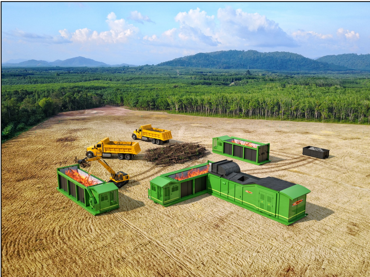
This portable 100kW Power Module powers all three FireBoxes, produces resalable BioChar and only requires one operator.
