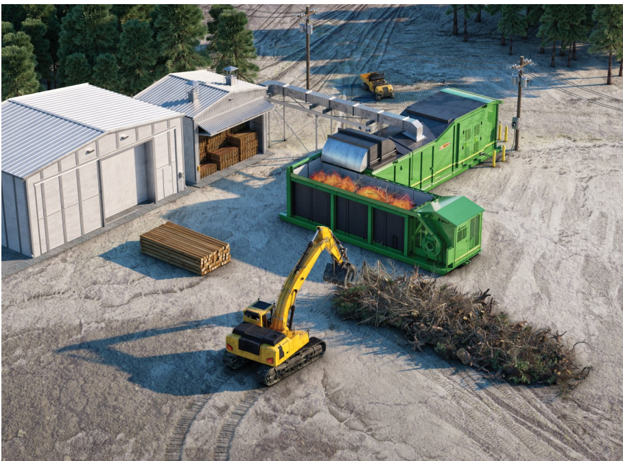
Example of thermal energy being used to supply a wood kiln for drying
